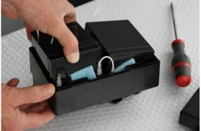
Use a small screwdriver to open the cover of the control box. Remove the batteries and unplug the connectors. Insert new batteries and reconnect them accordingly.
