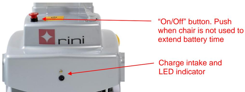
The "On/Off" button must be "On" during charging.
